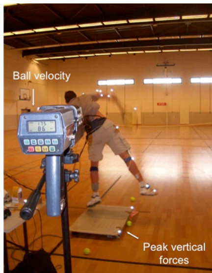
Figure 1. Peak vertical forces and post-impact ball velocity were determined by means of force platform and radar, respectively.
