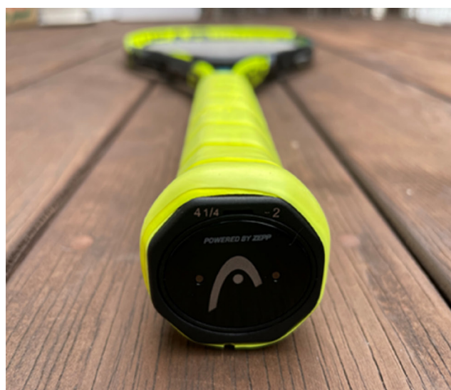
Figure 1. Tennis racket-mounted motion analysis sensor (HEAD Tennis Sensor; ZEPP).
