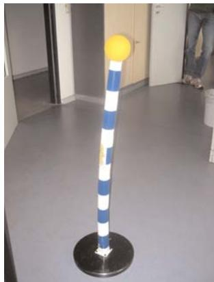
The ball pendulums or the pylons are located on each double court sideline. The distance between the two ball pendulums amounts exactly 11.0 m. Thus it is also possible to perform the test without a tennis court, if you measure a straight running track of 11.0 m. Two players can be tested simultaneously with one pair of ball pendulums. Up to 8 players can be tested at the same time on one court (Figure 2).
